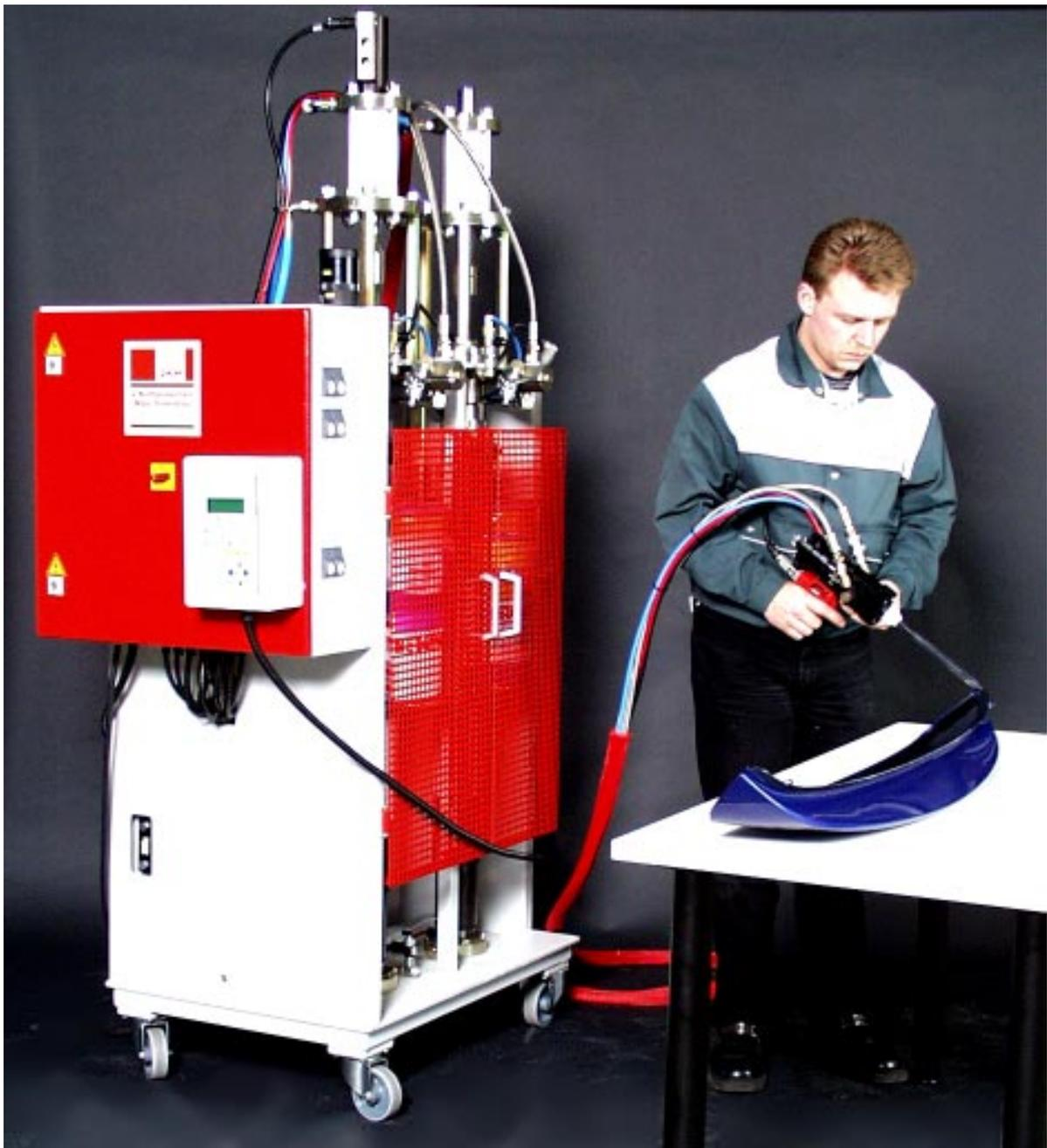
Metering Unit for Processing of Adhesives
